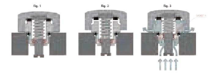
NOTE: To guarantee complete water-resistance, the valve crown must be screwed down tightly whenever the watch is immersed in water.
